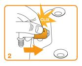
Set the safety slide to **OFF**, attach the connector to the NU® connection nozzle and then engage the solide in the **ON** position, thus activating the lock.
